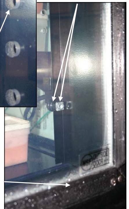
Additional view of Thumbscrew and Nut from Case Rear.
