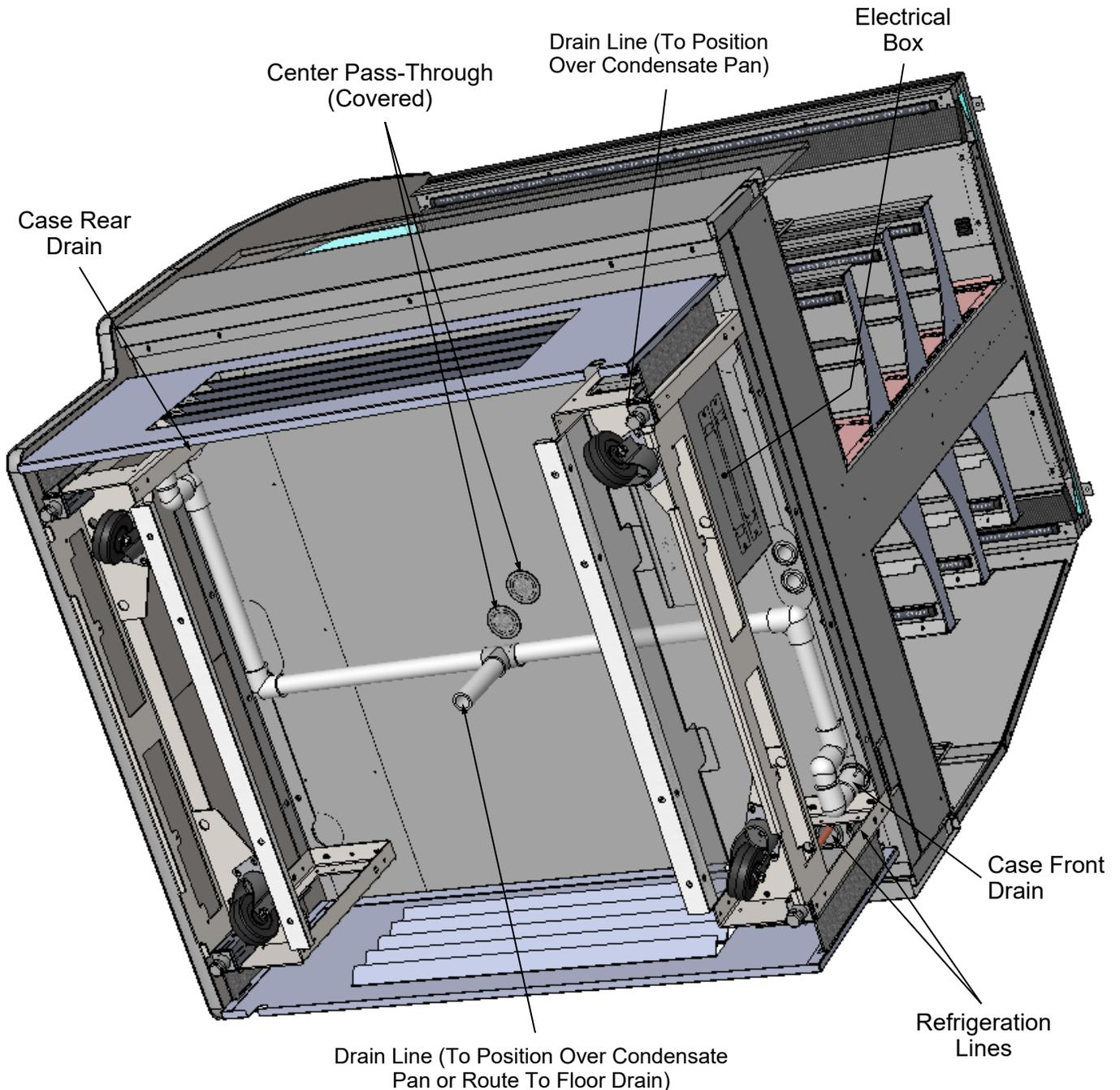
**Self-Contained Merchandiser's Condensate Unit Illustrated Parts Breakdown**
