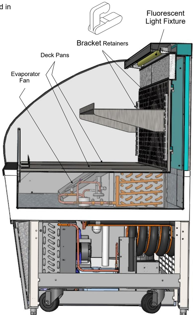
**Caution! Do not crimp or kink copper tubing while sliding condenser unit out from under case!**
